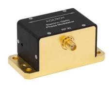
The GHz Resonant Optical Phase Modulator provides high speed free space optical phase modulation based on an electro-optical technology. It integrates a resonance electrical circuit inside the package to facilitate low driving voltage. The device can be driven by a function generator. It further integrated TEC temperature controller for stable operation.
